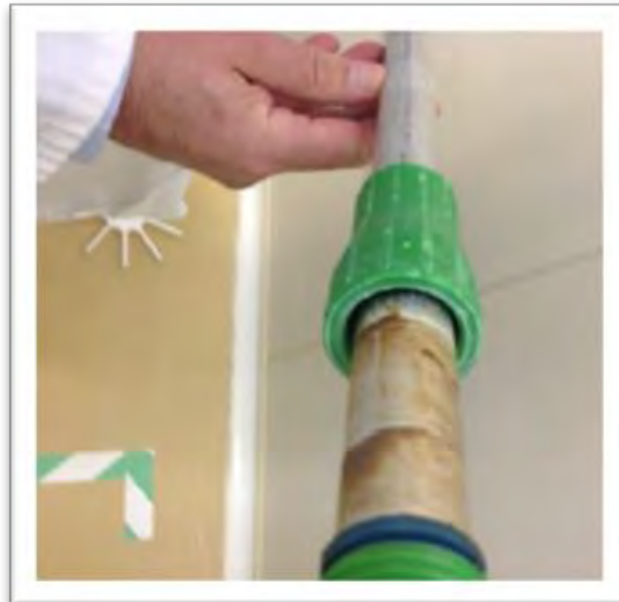
Contamination build-up under the screw thread handle fixing
